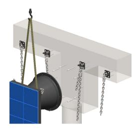
Determine the position of the rubber fenders, front panel, and accessories according to the shipping plan. Select suitable flat trucks, cranes, forklifts, hooks, and lifting slings for unloading. During the unloading process, please follow:
